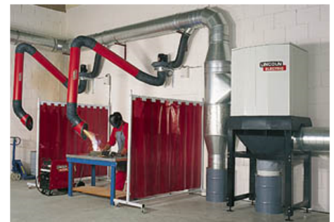
Figure 3. A low-vacuum high-volume source capture system.
