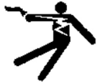
Figure 2. This symbol warns you about watching for electric shock when working.
