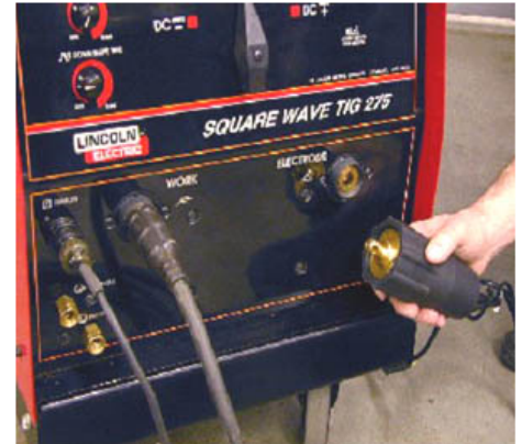
Figure 2. Make sure that all cables are installed in the welder properly.
