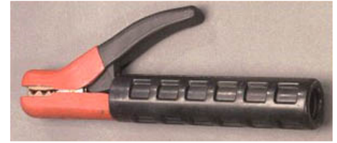
Figure 1. Like all arc welding components, the electrode holder must be dry and in good condition.
