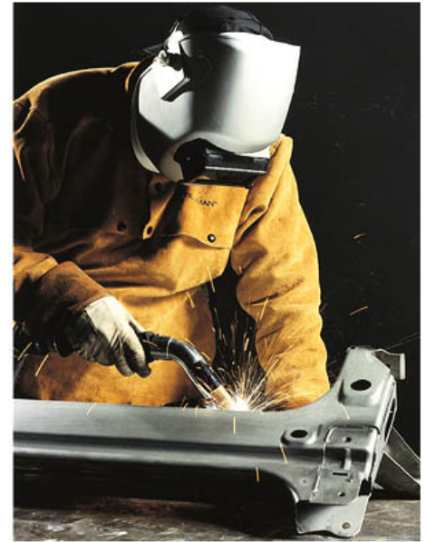
Figure 1. A properly dressed welder.
