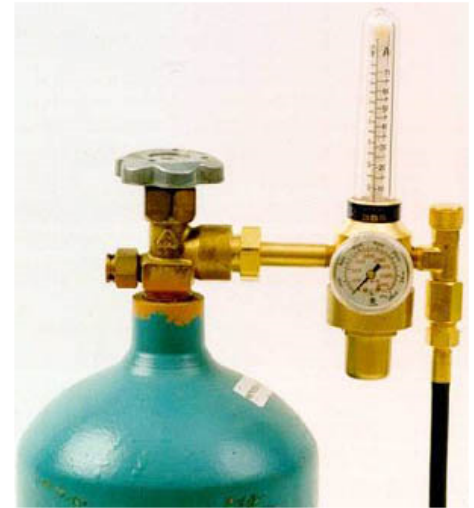
Figure 2. Welders must exercise caution when attaching a regulator to the shielding gas.
