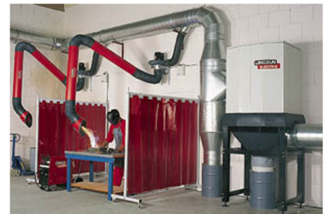
Figure 3. Appropriate ventilation protects the welder from harmful fumes.
