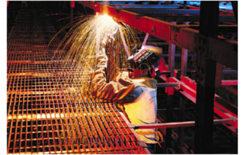
Figure 1. Spatter can quickly cause a fire if it contacts flammable or combustible material.
