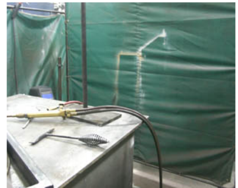
Figure 2. If you must weld in a cluttered or high-traffic area, use fire shields.
