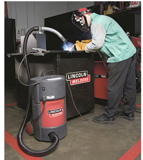
Figure 2. A high-vacuum low-volume source capture system.
