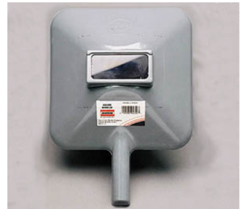
Figure 2. Hand-held face shields are commonly used by onlookers during a weld.
