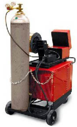
Figure 1. Gas cylinders must be secured to prevent explosion.
