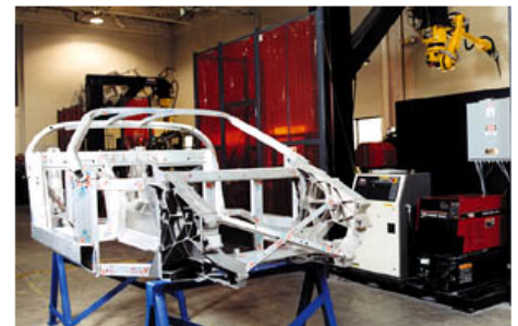
Figure 3. A welded aluminum car frame.
