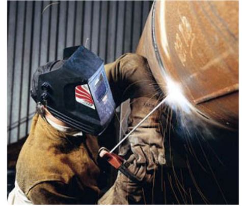
Figure 1. Arc welding is frequently used to join metals.
