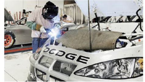
Figure 2. Performing gas metal arc welding on a racecar.
