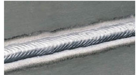
Figure 2. A weld bead created by gas metal arc welding.
