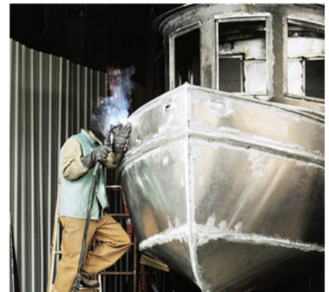
Figure 2. Welding an aluminum tugboat.
