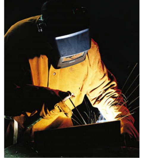
Figure 1. Arc welding uses electricity to generate heat and melt the metals.
