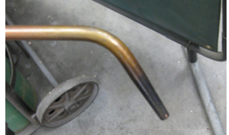
Figure 1. Welding tips may darken on the exterior with normal use.
