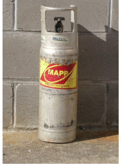
Figure 1. MAPP gas is an alternative to acetylene for oxyfuel welding.
