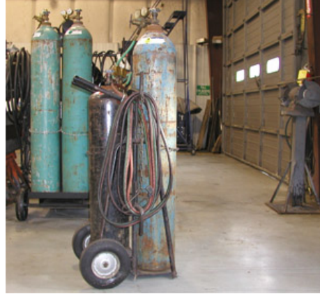
Figure 1. Visible wear to an oxyfuel outfit should be inspected before use. You should be certain the wear does not affect the safe operation of the outfit.
