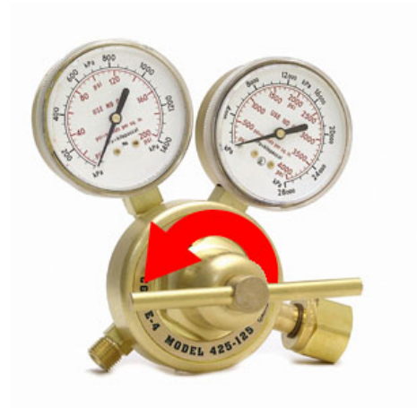
Figure 3. Turn the regulator screws counterclockwise until they are loose to complete shutting the torch off.
