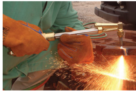
Figure 2. The intensity and brightness of the oxyfuel flame and the sparks it gives off can damage your eyes.
