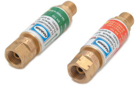
Figure 1. Flashback arrestors prevent the flame from moving up into the hoses and causing an explosion.
