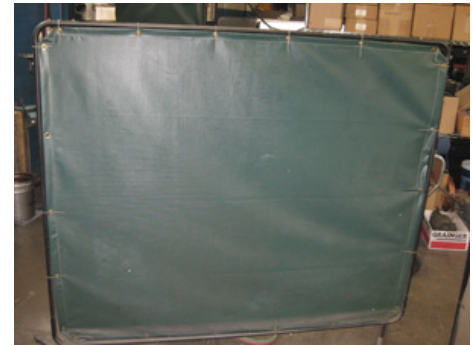
Figure 2. Fire shields prevent sparks from escaping the welding area.
