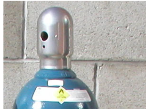
Figure 2. Valve caps should be kept on all cylinders when they are not being used.
