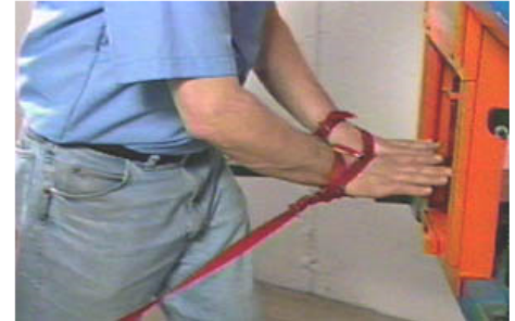
Figure 1. To keep employees' hands from getting caught in machinery, employers added wrist restraints.
