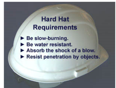
Figure 2. Hard hats must conform to these requirements.
