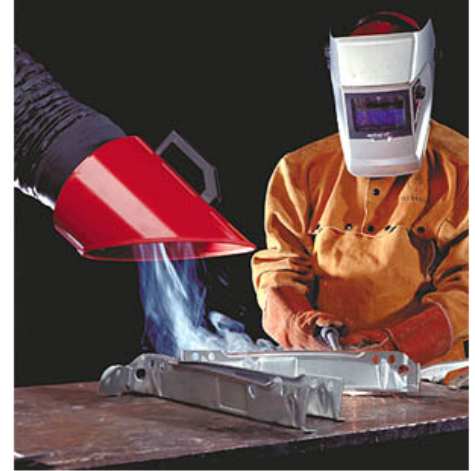
Figure 1. This coat and pair of gloves overlap to protect the employee's arms.
