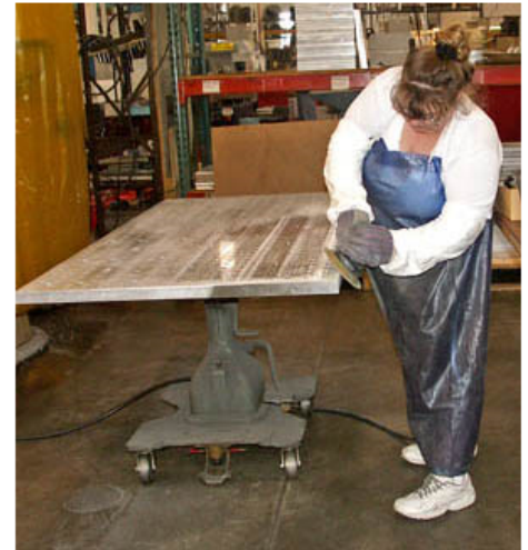
Figure 2. The apron worn by this employee is designed to repel liquids.
