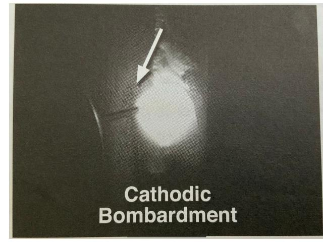
Because aluminum conducts heat 6x faster than steel, you must weld at higher amperages to compensate for the heat conducted away from the weld • Additionally, the rate of thermal expansion is about **2x** that of steel so you must be careful of distortion
