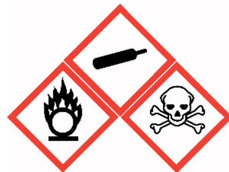
Figure 1. Three of the new pictograms for hazard identification: flammable (oxidizer), compressed gas, and toxic. The new symbols must have a diamond-shaped border in red.
