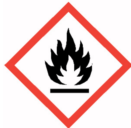
Figure 1. The GHS pictogram for fire hazard that will appear on labels and signs.
