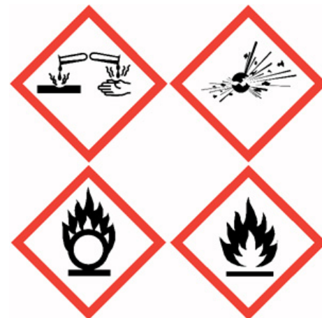
Figure 1. Corrosives, explosive chemicals, and flammable chemicals are considered physical hazards. Above are the GHS pictograms for these hazards.
