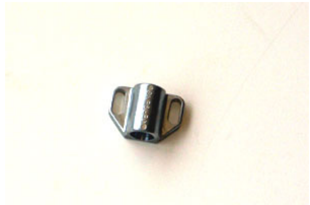
Figure 2. This spring stop component contains zinc and aluminum.
