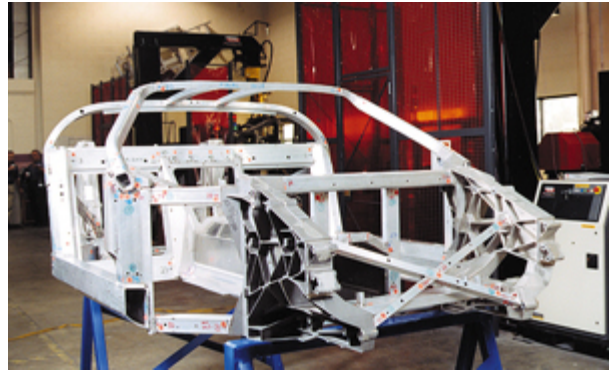
Figure 1. This aluminum car frame offers corrosion resistance.
