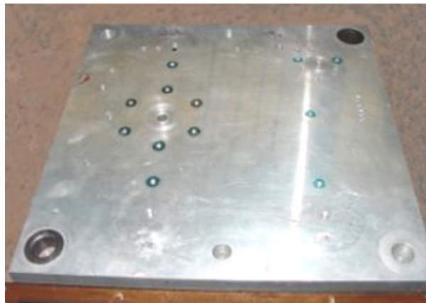
Figure 2. Lightweight aluminum plates are used to make workholding components.
