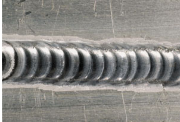
Figure 1. The film coating from this aluminum weld sample has been removed.
