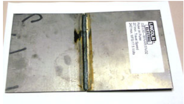
Figure 1. A galvanized steel weld.
