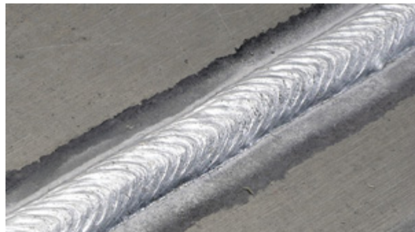
Figure 2. The thin gauge aluminum has been welded using GTAW.
