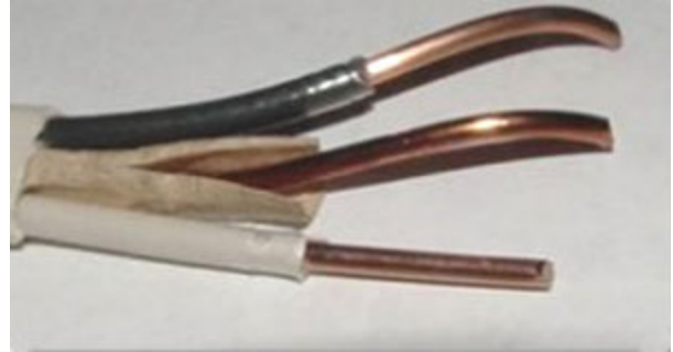
Figure 1. Copper wire is often used for electrical conductors.
