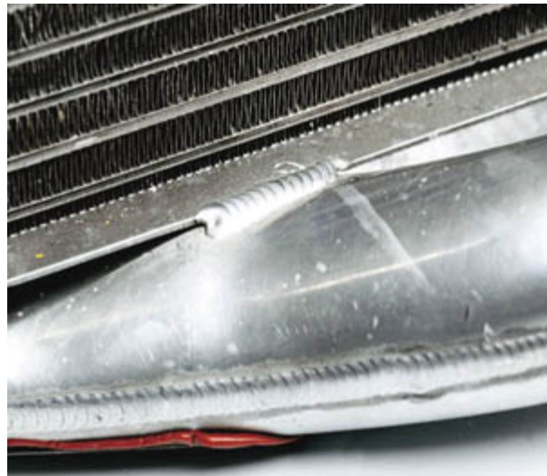
Figure 2. The thin gauge aluminum has been welded using GTAW.
