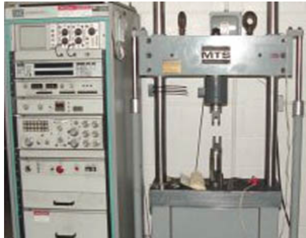
Figure 1. This machine tests a sample metal's strength by pulling it apart.
