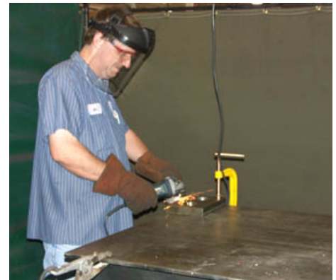
Figure 3. Fire shields are necessary to protect bystanders from applications that emit sparks.
