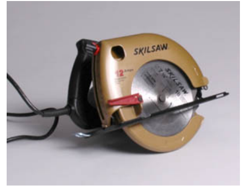
Figure 2. Safety guards must never be removed while a tool is in use.
