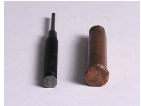
Figure 3. These tools have "mushroomed heads" as a result of frequent use and must not be used anymore.
