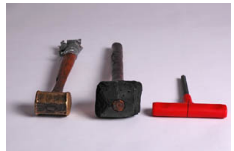
Figure 3. The handles and tools in these examples pose a safety risk, so the tools must be discarded.
