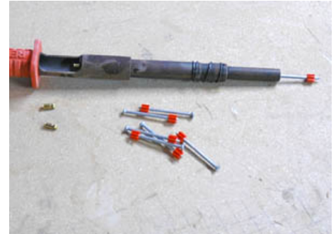
Figure 1. Powder tools pose so many safety risks that only approved personnel may operate them.
