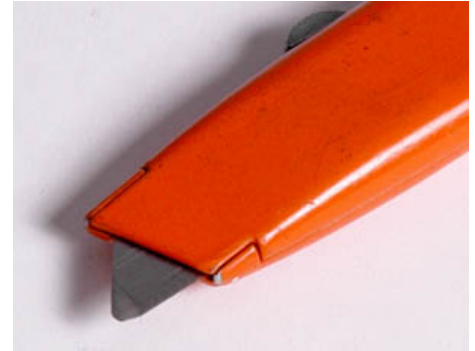
Figure 1. Using a dull blade like this one is a safety risk.
