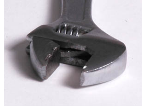
Figure 1. Do not use wrenches with damaged jaws.
