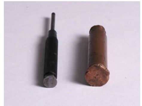
Figure 2. These tools have "mushroomed heads" as a result of frequent use and must not be used anymore.
