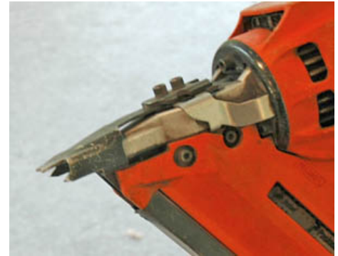
Figure 2. This pneumatic nail gun has a safety device so that nails are not ejected by accident.
