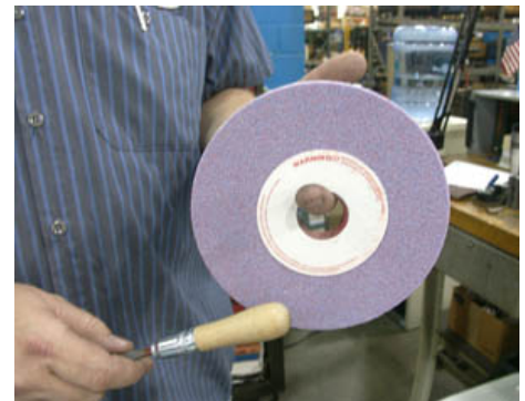
Figure 3. If the abrasive is cracked or damaged, you will hear a "dead" sound. If it is not defective, you will hear a ringing sound.
