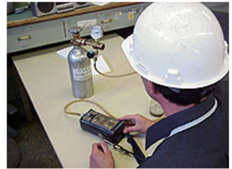
Figure 1. The entry supervisor must make sure that all preparations, such as calibrating atmospheric testing equipment, are performed prior to anyone entering the space.
