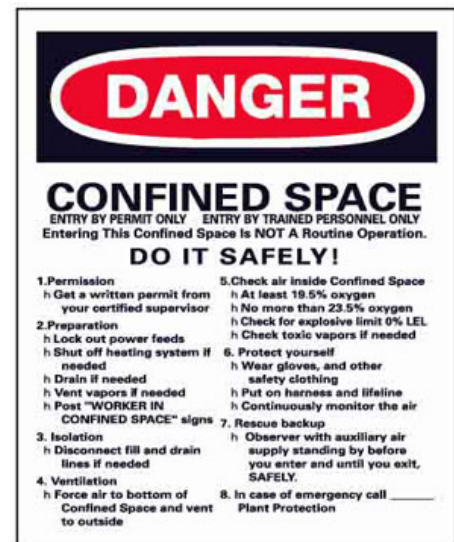
Figure 1. Proper work practices are vital for keeping employees safe in confined spaces. (Courtesy of NMC.)
