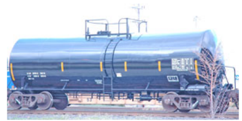
Figure 1. A rail car storage tank is considered an open-top confined space.
