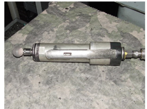
Figure 2. The tools you use within a confined space can cause physical hazards, such as the noise and vibration that can be caused by this hand-held grinding tool.
