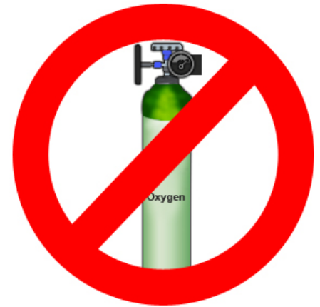
Figure 1. Oxygen use in confined spaces is a fire and explosion hazard, so it should never be used to purge the atmosphere.
