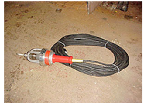
Figure 2. Confined spaces require special lighting, such as this explosion-proof utility light.
